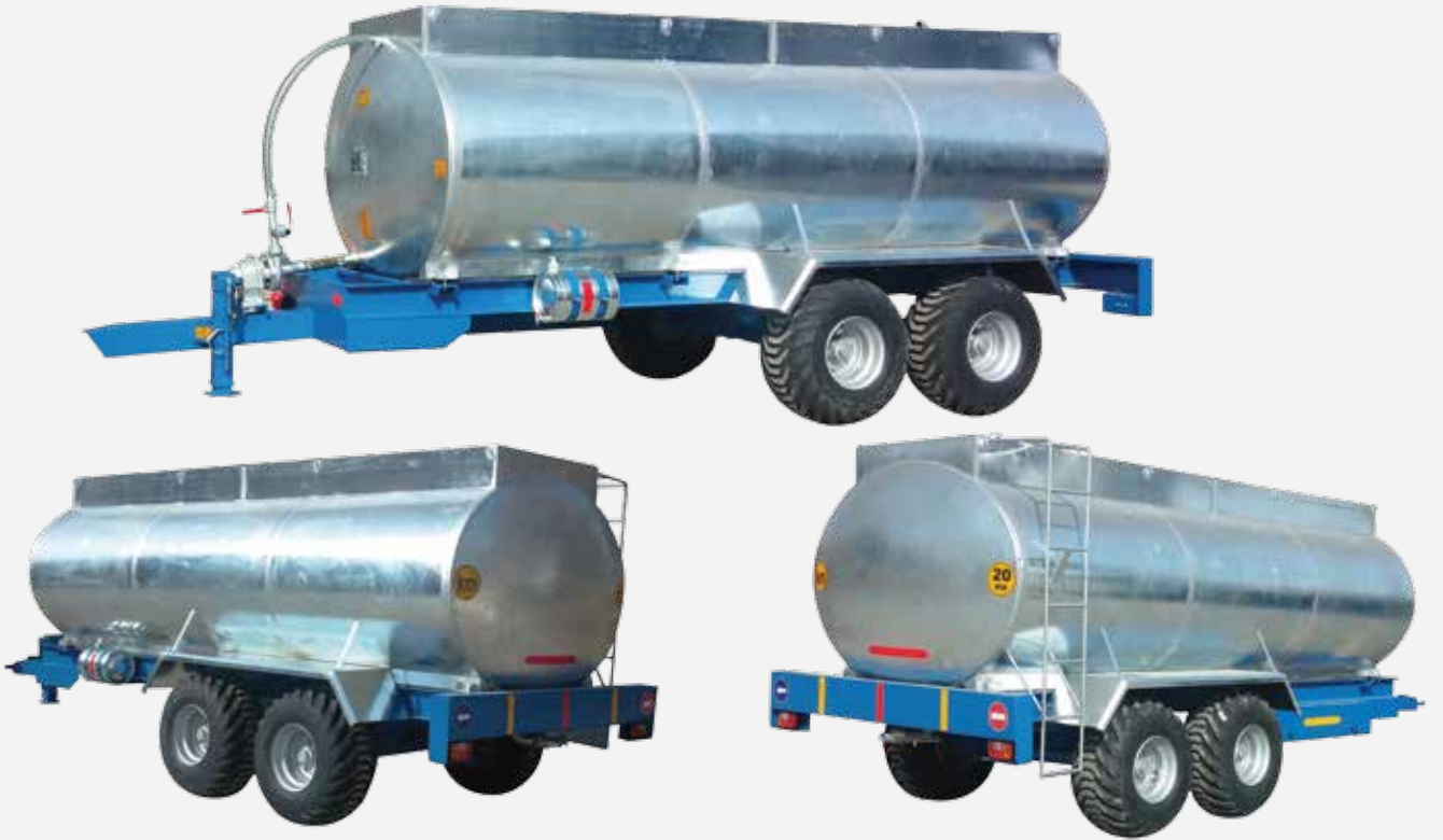
8 Ton Parabolik Dorse Tipi Santrifüjli Su Tankı / 8 Tons Parabolic Dorse Type Centrifugal Water Tank
